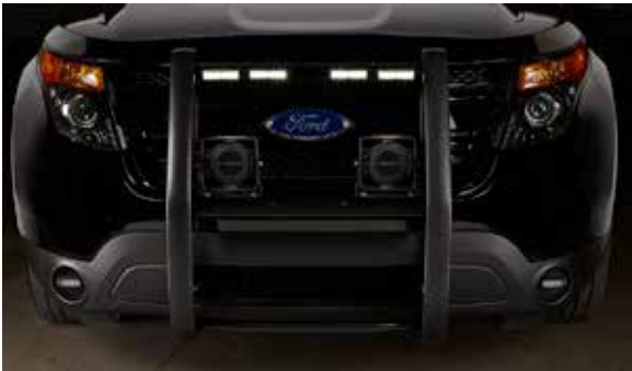
(2) ES100 Speakers mounted on the grille of a Ford® Interceptor
